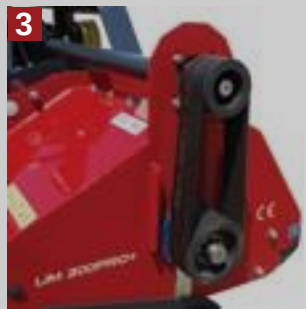
LATERAL TRANSMISSION via a set of special V-belts; Automatic spanning
