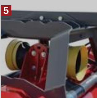
GEARBOX with two output shafts for front and rear attachment
