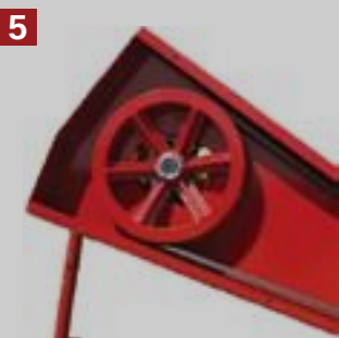
A SET OF V-BELTS transmits power to cutter bar driveline.
