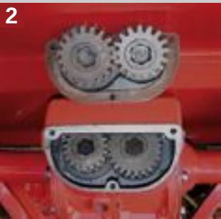
GEARBOX Four speed gearbox with two pairs of gear wheels
