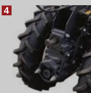
TWO OUTPUT SHAFTS optional for models FPM 410/414
