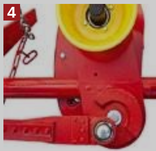
FRAME: Safety system for automatic release of the cutter bar in case of obstacle impact;
