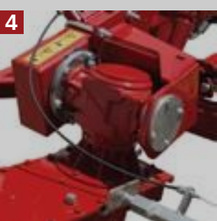
REINFORCED TRANSMISSIO N The gearbox is protected against collisions with obstacles
