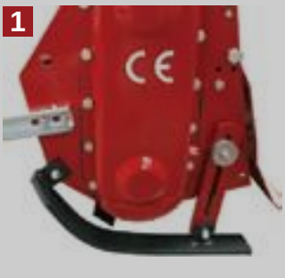
WORKING DEPTH ADJUSTMENT with help of side sliders
