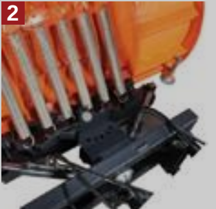
SHOCK AMORTIZ. SYSTEM when encountering an obstacle
