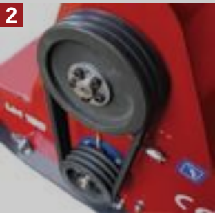
LATTERAL TRANSMISSION through toothed V-belts
