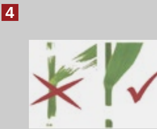
CUTTER BAR: a) Serrated knives for difficult working conditions; b) Reciprocating movement of cutter bars (Busatis system) provides precise, scissor-like cutting (without ripping) and contributes to faster plant regeneration and growth. c) Main bar is made of special type of steel (spring steel), offering high strength and appropriate flexibility.
