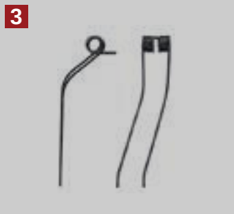
COLLECTING ELEMENTS made of high-quality spring wire
