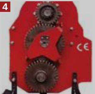
TRANSMISSION Gear drive transmission in oil bath
