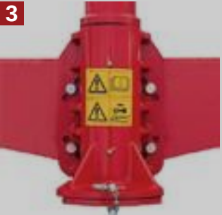
SNOWPLOUGH MOUNTING BRACKET: Horizontal angular adjustment of snowplough, and possibility of 360 degree rotation
