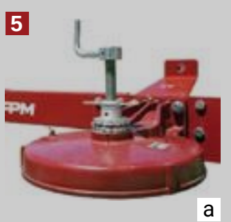
WORKING HEIGHT ADJUSTMENT: a) by adjusting gearbox height;
