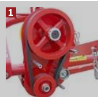
TRANSMISSION through V-belts with belt tensioners.
