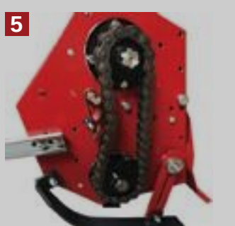
TRANSMISSION Chain drive transmission in oil bath
