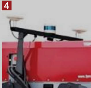
AUTONOMOUS DRIVING along pre-defined paths and GPS/RTK coordinates
