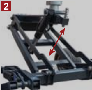
HYDRAULIC CYLINDERS X for raising to transport and lowering to operating position
