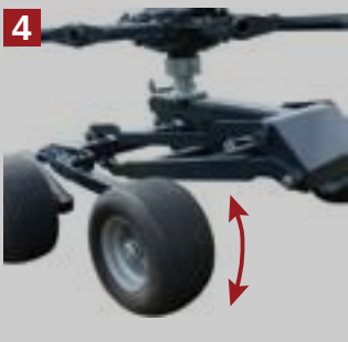
LEVERAGE SYSTEM for regulating lift and mowing height
