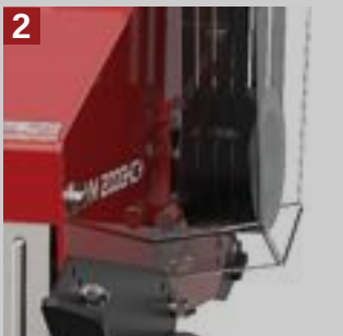
LATERAL TRANSMISSION through toothed V-belts
