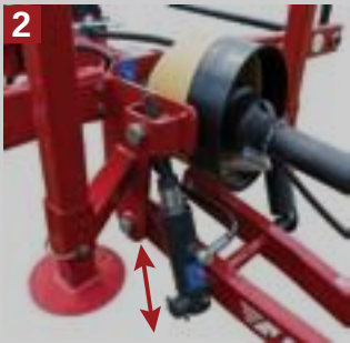
HYDRAULIC CYLINDERS X for raising to transport and lowering to operating position
